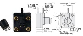
Electrical Rating: 60 ma. AC resistive 40 ma. DC resistive @ 120 volts
